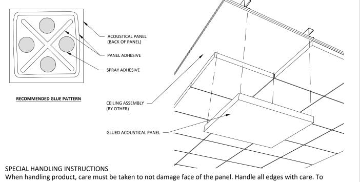
avoid damage, do not twist or bow the panels during installation.
