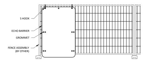
To secure Echo Barrier to fencing, thread cable- or bungee-ties (sufficiently strong) through Echo Barrier eyelets to the supporting structure. Eyelets should adjoin each other when barriers overlap, which is recommended for best noise attenuation results.
