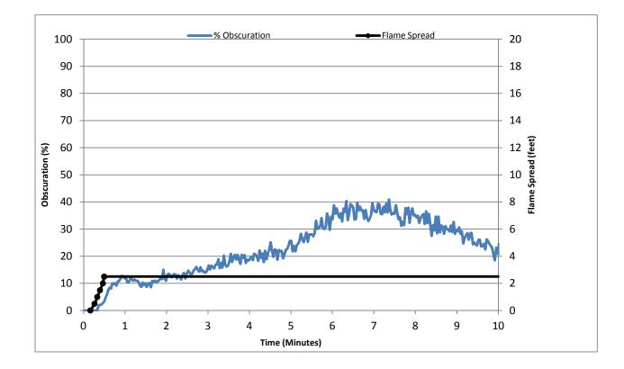
Test Num.: 4 R8078 / 4786322820 03281412 Flame Spread Index:10Smoke Developed Index:300Max. Flame Spread (ft.):2.5
