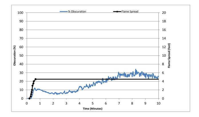
Test Num.: 5 R8078 / 4786322820 03281413 Flame Spread Index:20Smoke Developed Index:250Max. Flame Spread (ft.):4.5
